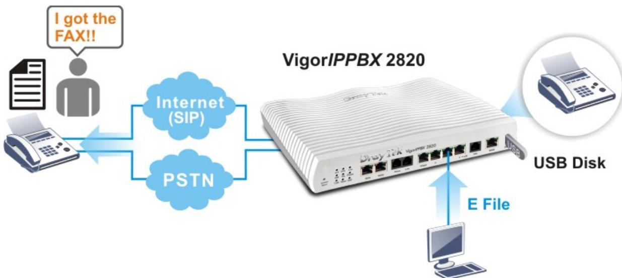
In addition, virtual FAX can be used to receive the document sending from remote end through Internet (SIP) or PSTN line. VigorIPPBX 2820's built in FAX machine will save the document from the sender as a file and store in USB Disk. Later, VigorIPPBX 2820 series will send an e-mail attached with the file to the receiver.
